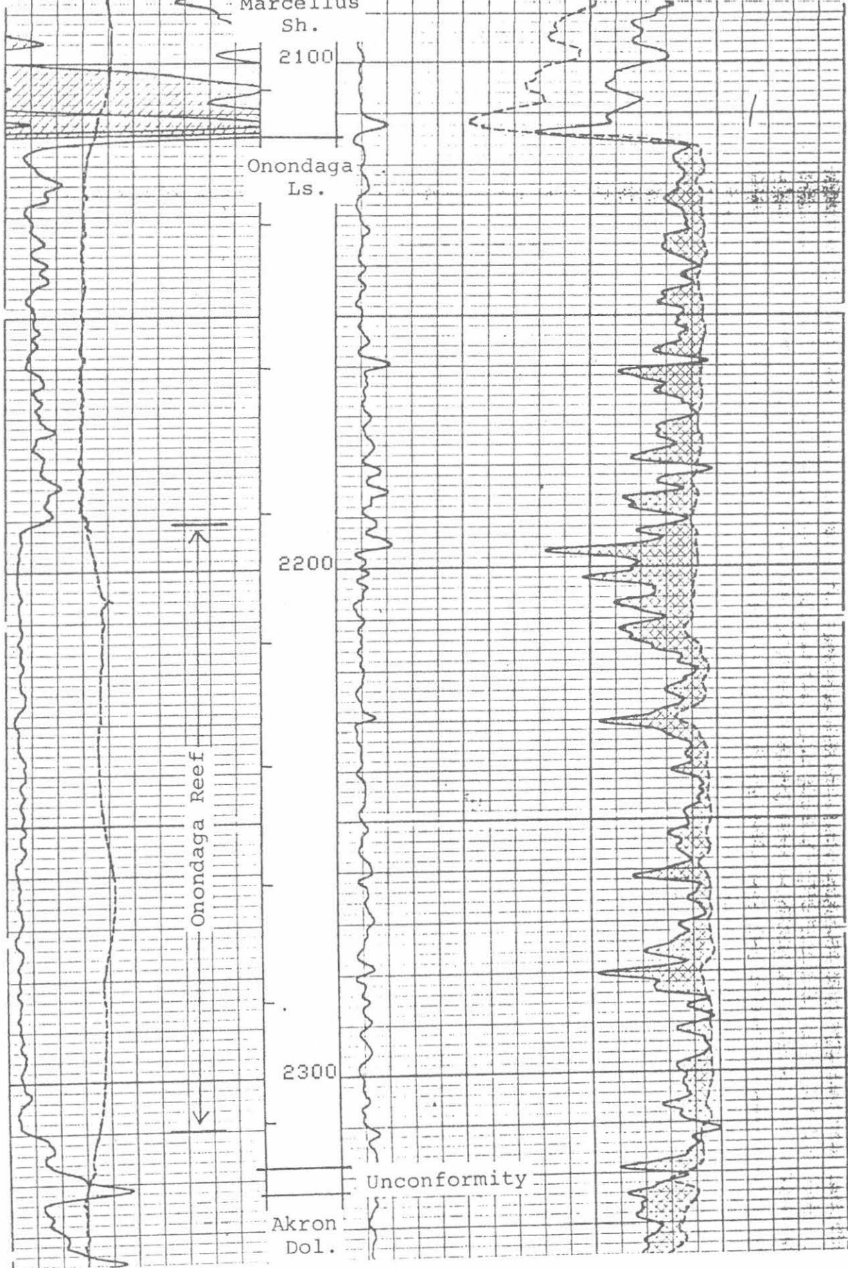
Figure 4. Geophysical log of an Onondaga bioherm in the L. Philips #1, drilled by Empire Exploration, Inc., in the Town of Villenova, Chautauqua County, N.Y.
